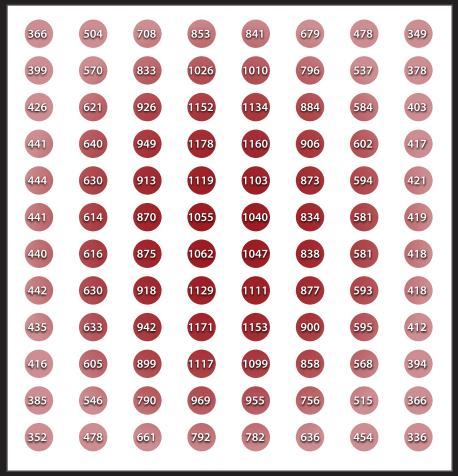
**Note:** Photosynthetic Photon Flux Density (PPFD) data is produced by using professional lighting simulation software and third party laboratory photometric files. All PPFD data are measured in µmol/s/m². The result assumes a single fixture being mounted in a 4'x4' grow tent with 85% wall reflectance. Actual measurement may vary depending on actual use conditions, input voltages, and measuring instruments. Professional lighting plans for commercial applications are available upon request.
