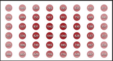
**Note:** Photosynthetic Photon Flux Density (PPFD) data is produced by using professional lighting simulation software and third party laboratory photometric files. All PPFD data are measured in µmol/s/m². The result assumes a single fixture being mounted in a 4'x4' grow tent with 85% wall reflectance. Actual measurement may vary depending on actual use conditions, input voltages, and measuring instruments. Professional lighting plans for commercial applications are available upon request.
